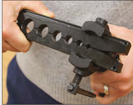
Railing allows yoke to smoothly travel while keeping the flaring tool and bar aligned
