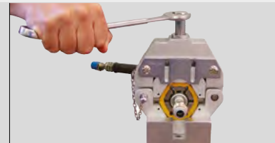
Close yoke, insert pin and turn arbor screw
